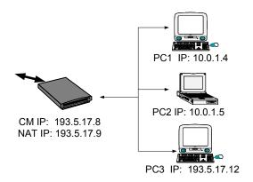
Figure 2 presents a home network with three PCs. It assumes an HA with embedded PS (i.e. a cable modem with firewall/NAT functionality). PC1 and PC2 both have local IP addresses that were received from the DHCP server located inside the CM. PC3 gets its IP address from the DHCP server at the Head End. It is an address outside the scope of the home.
