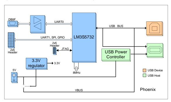
Figure 1. Phoenix USB Test Board Block Diagram
