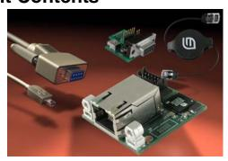
The Stellaris® Serial-to-Ethernet Module is offered as a stand-alone, ready-for-production module (MDL-S2E) and also as a reference design kit (RDK-S2E). The RDK ships with everything needed to quickly evaluate and easily customize the MDL-S2E for your specific application, including:
