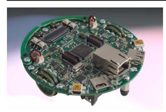
The Stellaris® LM3S9B92 EVALBOT Robotic Evaluation Board (EVALBOT) is a robotic evaluation platform for the Stellaris LM3S9B92 microcontroller. The board also uses a range of Texas Instruments' analog components for motor drive, power supply, and communications functions. After a few minutes of assembly, the EVALBOT's electronics are ready-to-run.
