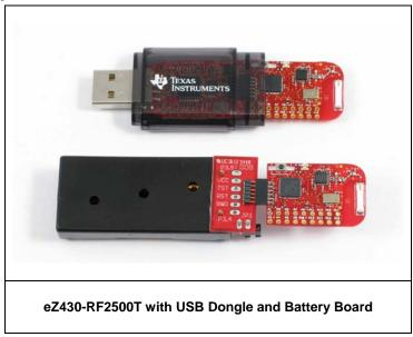
The Stellaris 2.4 GHz SimpliciTI Wireless Kit includes two eZ430-RF2500T boards. These can be powered either via a USB dongle or battery board, both of which are provided in the kit. The boards are pre-programmed as end devices for the "Access Point as Data Hub" SimpliciTI example application.
