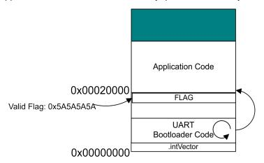
Figure 5. UART Bootloader Jumps to Application Code
