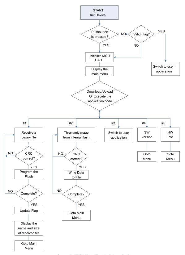
Figure 1. UART Bootloader Flowchart
