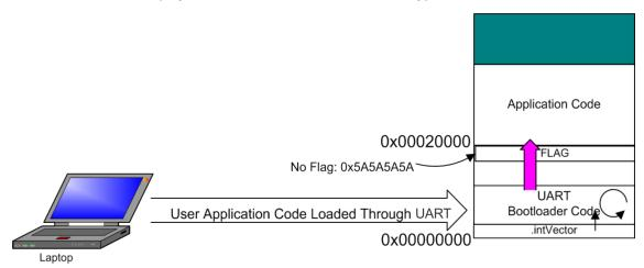
Figure 4. User Application Code is Loaded Through the UART Bootloader
