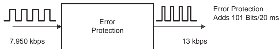
Figure 7. Error Protection Adds 101 Extra Bits per Speech Frame
