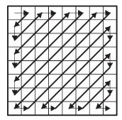
Figure 3. H.261 Recommended Zig-Zag Scanning Procedures
