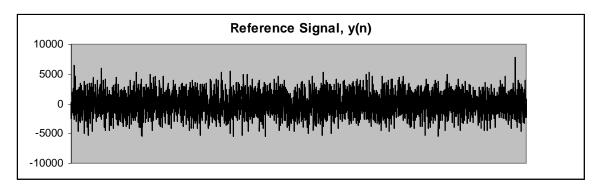
The reference input signal represents 4000 samples (0.5 sec) of band-limited white noise. The echo signal is the reference signal passed through a digital filter with 32 samples flat delay, a total of 50 taps and 10dB loss. This filter simulates the response of a hybrid in a telephone network.
