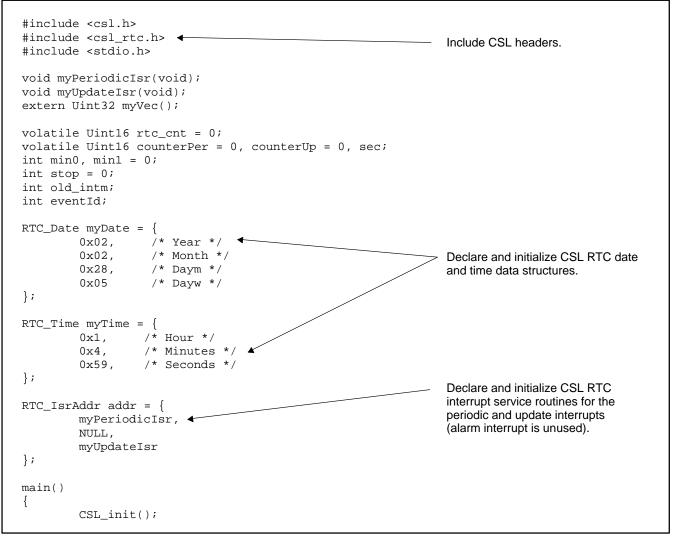
Figure 8. Example 3: CSL RTC Interrupt Dispatcher Code
