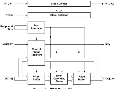
Figure 1. RTC Block Diagram
