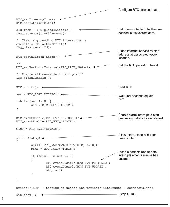
Figure 8. Example 3: CSL RTC Interrupt Dispatcher Code (Continued)
