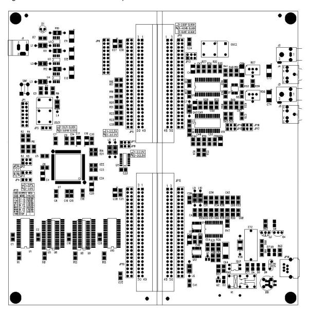
Figure 29. TMS320C548/9 Development Board Placement
