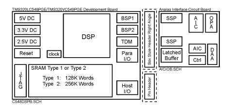
Figure 17. TMS320C548/9 DSP Board
