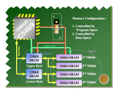
The TMS320C548/9 DVB 128K-word (Type 1) or 256K-word (Type 2) external memory is determined while the components are mounted (see Figure 6). The memory should be very high-speed asynchronous SRAMs.
