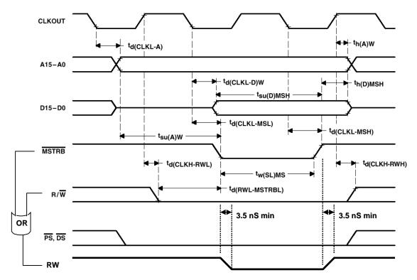
Figure 10. SRAM Write Timing
