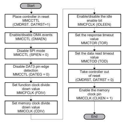
Figure 5. MMC Controller Configuration Configuration (MMC\_initNative)
