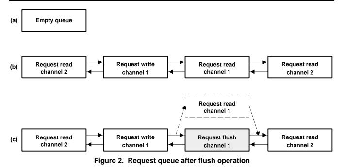
The driver waits until the pending write operation on channel 1 is completed before it returns the flush call.
