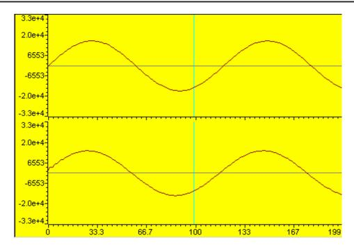
Figure 8. IIR Filter Passband Input (top) and Output (bottom)
