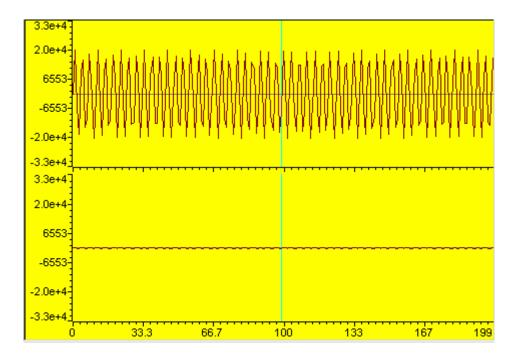
Figure 6. FIR Filter Stopband Input (top) and Output (bottom)
