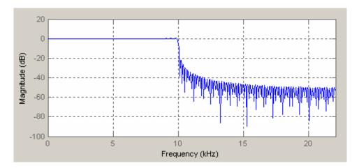
Figure 4. Frequency Response of a Low-Pass FIR Filter
