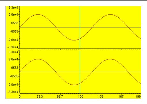
Figure 5. FIR Filter Passband Input (top) and Output (bottom)
