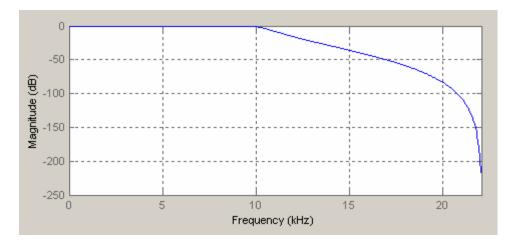
Figure 7. Frequency Response of a Low-Pass IIR Filter
