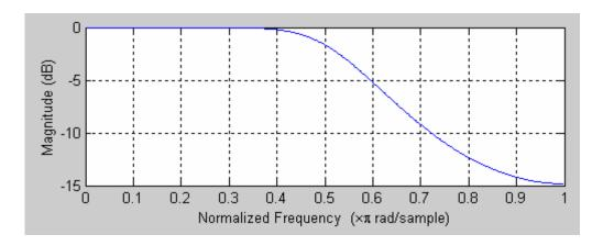
Figure 10. Low-Pass IIR Lattice Filter Frequency Response
