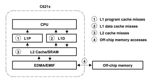
Figure 2. C621x Memory Hierarchy and Potential Overhead
