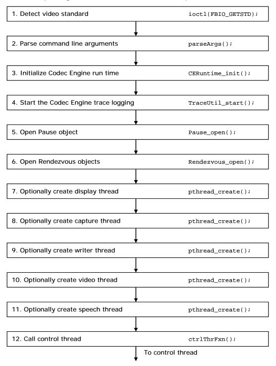
Figure 3. Main Thread Flow
