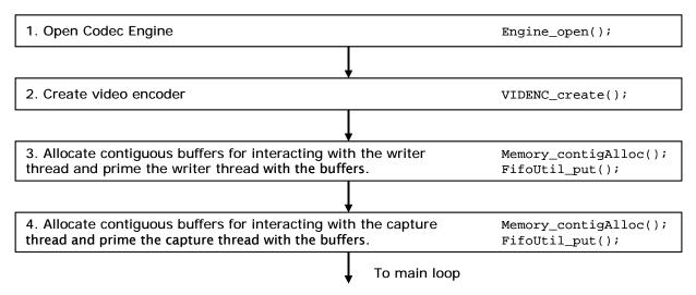
Figure 6. Video Thread Initialization Flow
