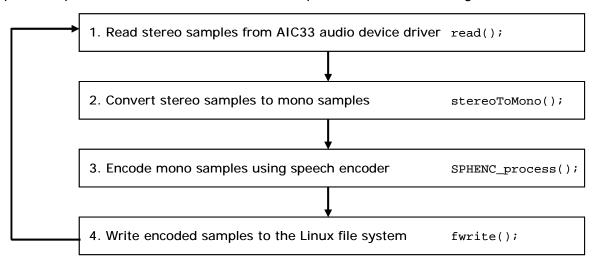
Figure 5. Speech Thread Main Loop Flow
