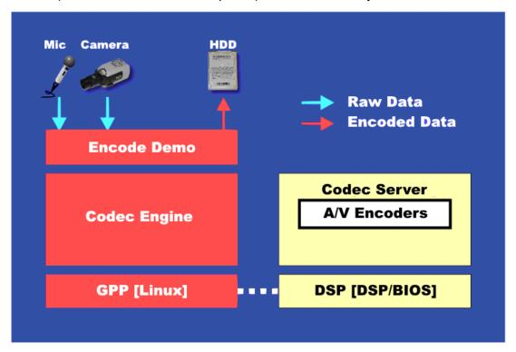
Figure 1. Encode Demo Architecture
