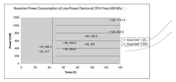
Figure 2. Baseline Power Consumption Across Voltage and Temperature: Low-Power
