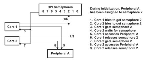
Figure 2. Example of Two CPUs Trying to Access the Same Peripheral
