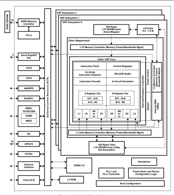
Figure 1. C6474 Block Diagram
