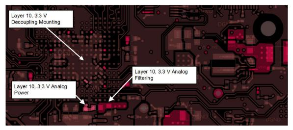
Figure 12-9. AM263x controlCARD Excerpt – Common 3.3 V Plane Transition Vias
