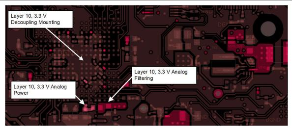
Figure 12-11. AM263x controlCARD Excerpt – 3.3 V Digital and Analog Power Decoupling Mounting, Layer 10
