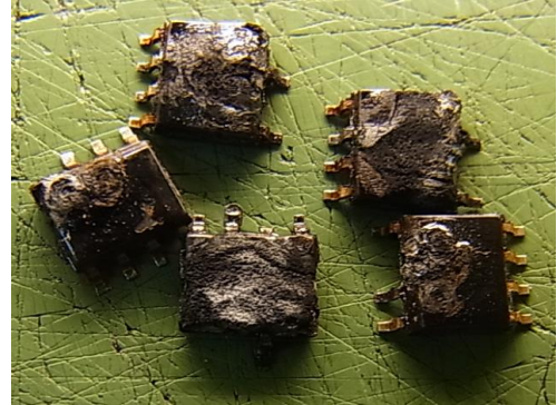
carbonized mold compound
