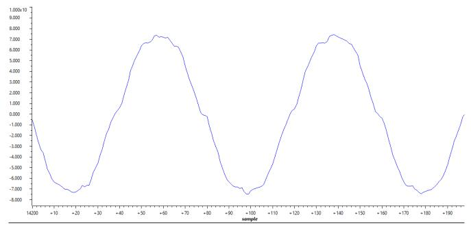
Figure 2-36. Phase A Current Open Loop
