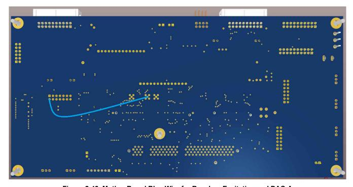
Figure 2-43. Mother Board Blue Wire for Resolver Excitation and DAC-A
