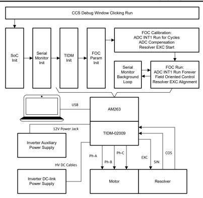
Figure 1-2. Traction System Diagram
