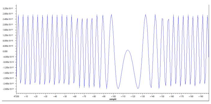
Figure 2-47. Resolver Sine Envelope for a Transition from Forward to Backward
