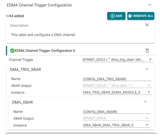
Figure 2-30. EDMA Channel Trigger Configuration
