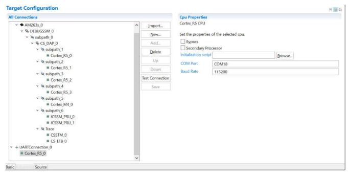
Figure 2-10. Update CPU Properties in Advanced Target Configuration
