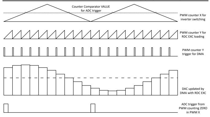
Figure 2-41. Software Resolver Synchronization and Excitation
