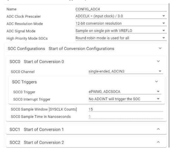
Figure 2-26. ADC4 SOC Configuration
