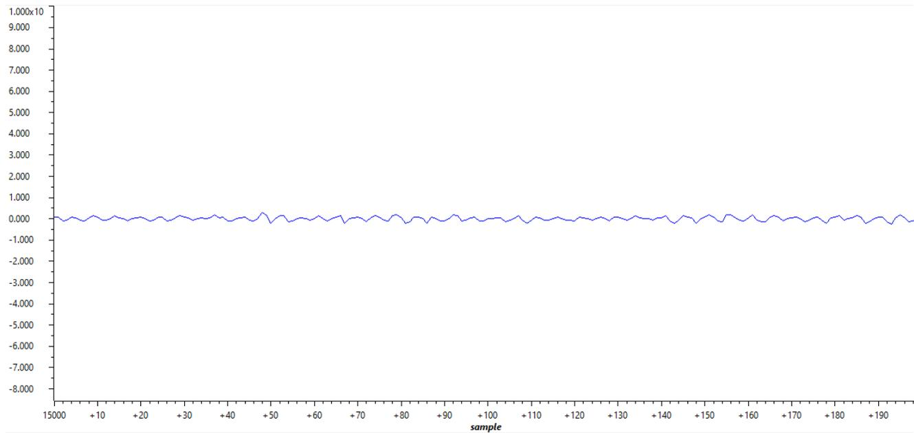
**Figure 3-18. Plotted Phase A Current at No Load**
