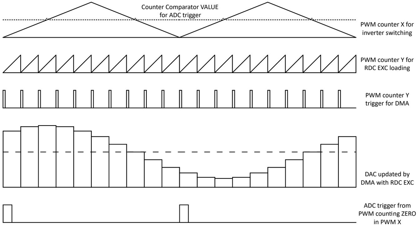
**Figure 3-25. Software Resolver Synchronization and Excitation**
