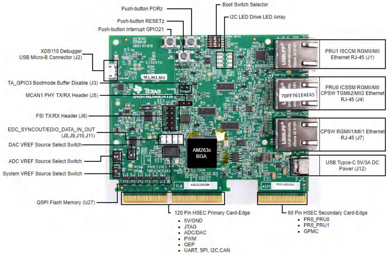
**Figure 3-1. User Interfaces of AM263x Control Card**
