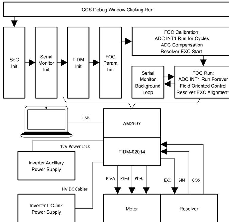
**Figure 2-3. Traction System Diagram**
