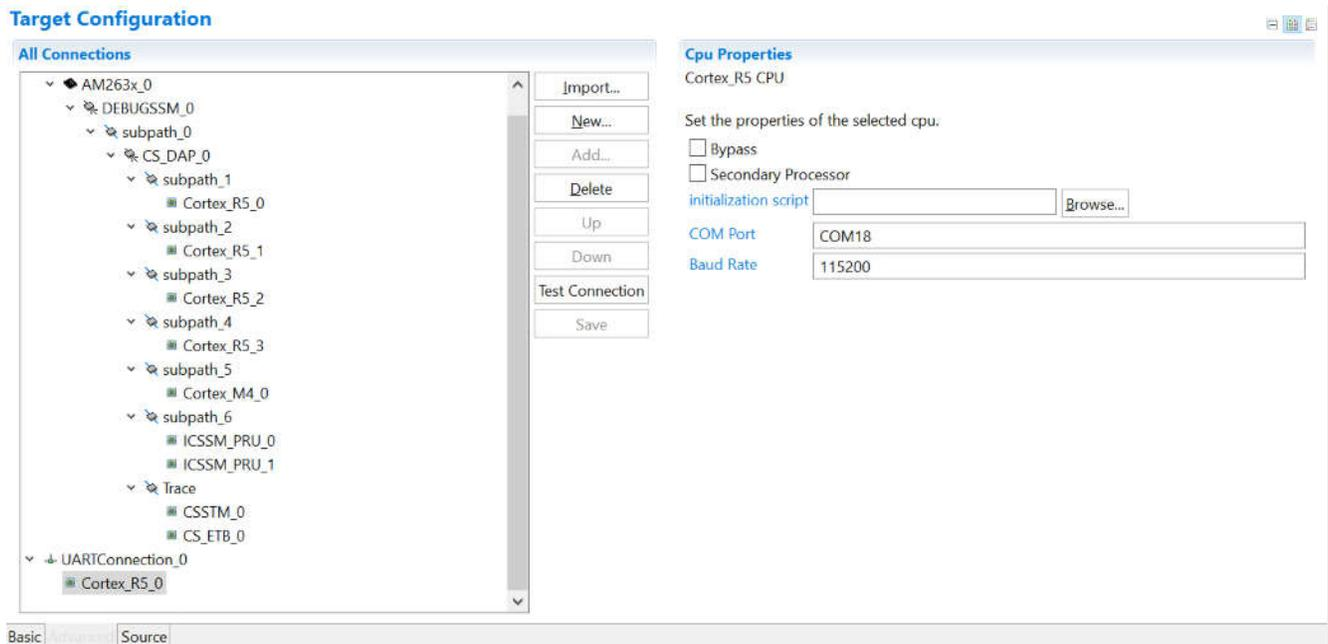
Figure 3-10. Update CPU Properties in Advanced Target Configuration
