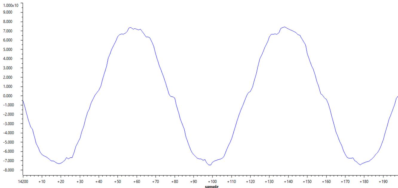
Figure 3-20. Phase A Current Open Loop
