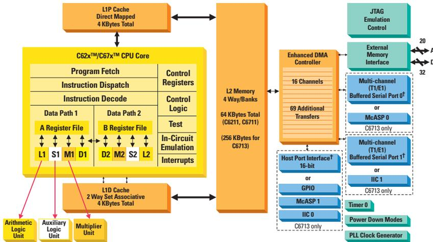
The C6713 DSP offers the audio customer base unparalleled levels of flexibility and performance. This superset of the C6711 and C6712 DSPs includes I<sup>2</sup>S, I<sup>2</sup>C and S/PDIF transmit support as well as enhanced memory space. Non-audio customers can also use this DSP as an upward migration path from the C6711 DSP.
