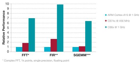
\*\* Complex block FIR, single precision, floating point, 128 samples, 16 coefficients
