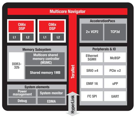
▲ Figure 1: TMS320C6657 block diagram
