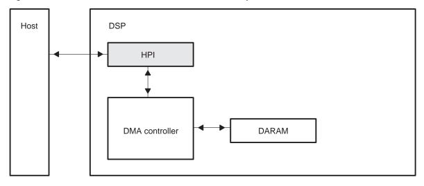
Figure 1. The Position of the HPI in a Host-DSP System
