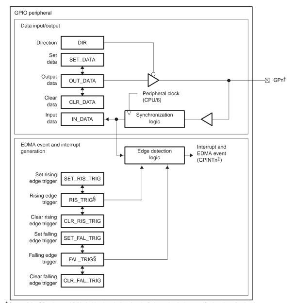
Figure 2. GPIO Peripheral Block Diagram
