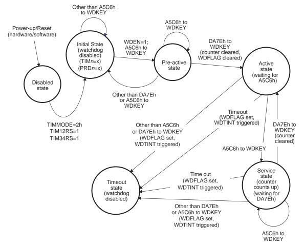
Figure 10. Watchdog Timer Operation State Diagram
