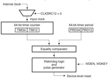
Figure 9. Watchdog Timer Mode Block Diagram
