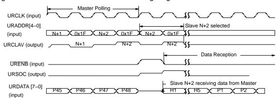
Figure 6. ATM Controller Slave Receive Timing Diagram
