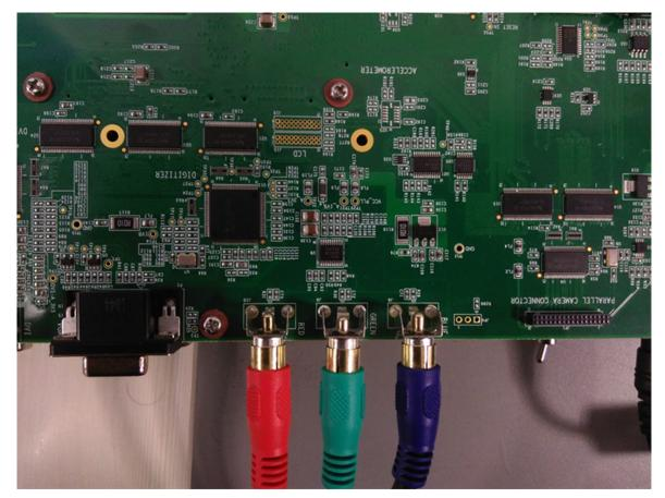
Figure 3. Analog Component Cable Connected to EVM
