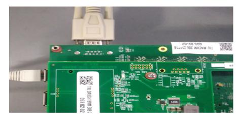
Figure 4. Serial Cable Connected to EVM
