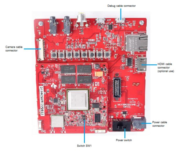
Figure 2. DM8127 CSK Connections (1 of 2)
