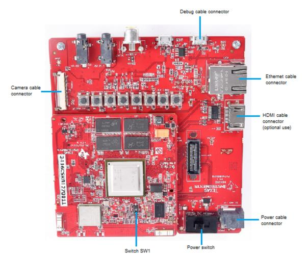
Figure 4. DM8127 CSK Connections (2 of 2)
