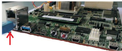
3. Insert DC-in cable to apply 12 V power.
