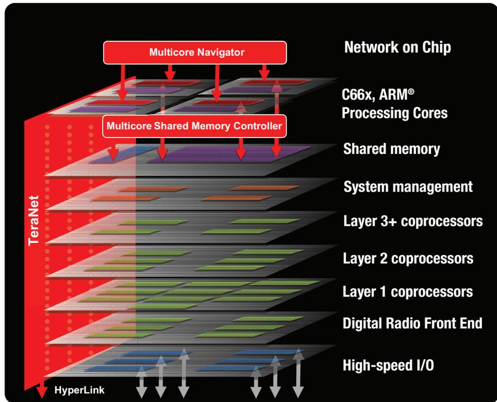
▲ **Figure 2.** TI's multicore SoC architecture.
