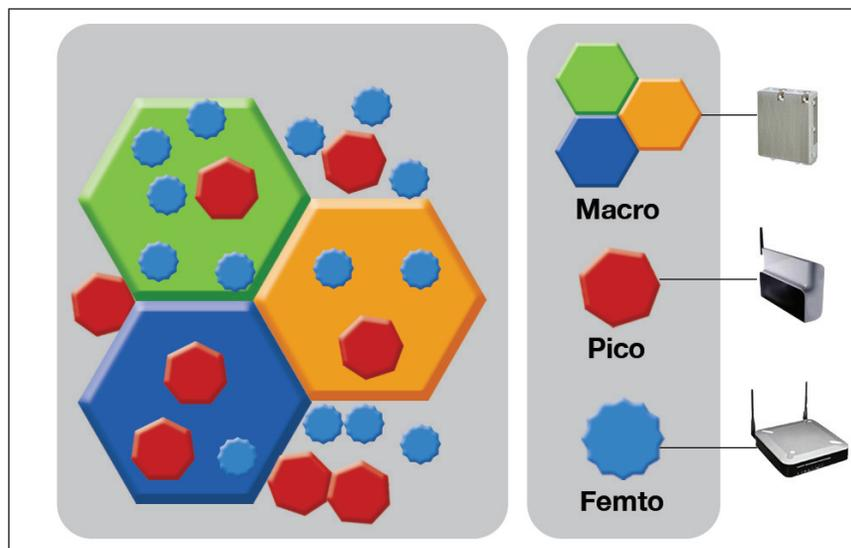
▲ **Figure 1.** *Impact of small cells on network architecture*
