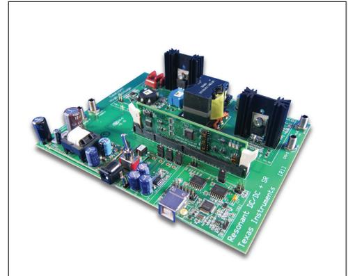
▲ Fig. 3b –Isolated LLC Resonant DC/DC Kit
