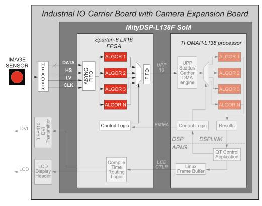
Figure 1. Image processing in Xilinx FPGA
