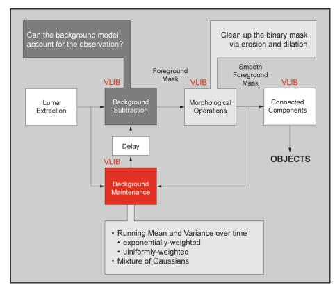
Figure 5. Moving object segmentation
