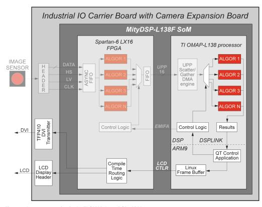
Figure 4. Image processing in the TI OMAP-L138 DSP+ARM9 processor
