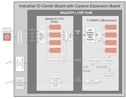
Figure 2. uPP Interface between the TI OMAP-L138 DSP+ARM9™ processor and an FPGA
