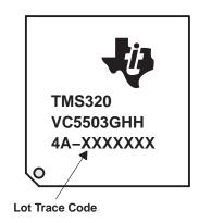
Figure 2. Example Markings for VC5503, GHH Package, Revision 1.0
