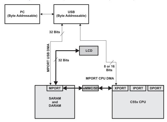
Figure 2. CPU, USB, LCD, and eMMC/SD Data Paths
