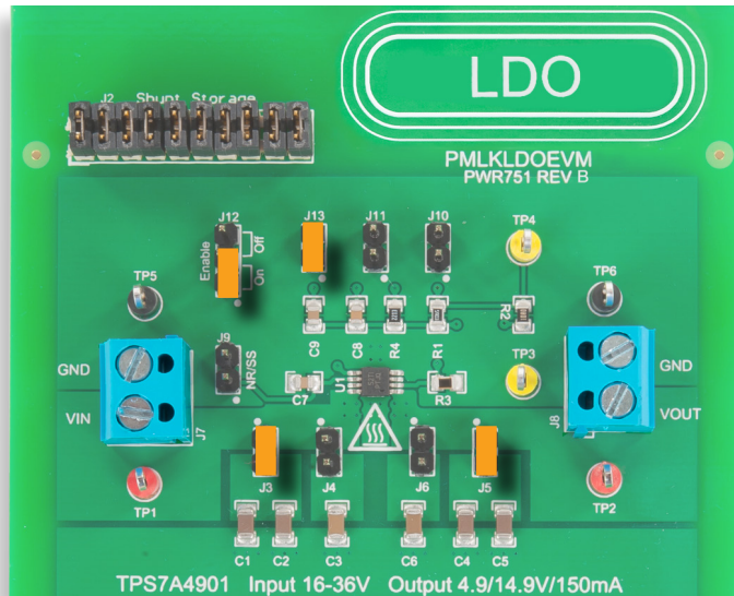
Figure 7. TPS7A4901 LDO board: jumpers set-up for Test#2
