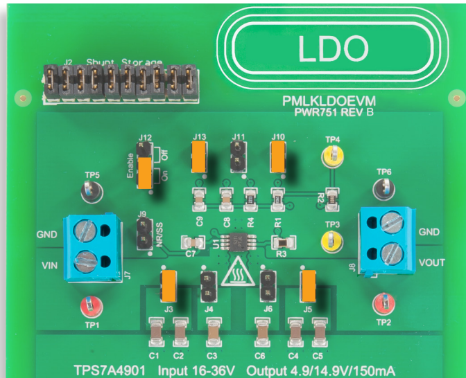
Figure 6. TPS7A4901 LDO board: jumpers set-up for Test#1
