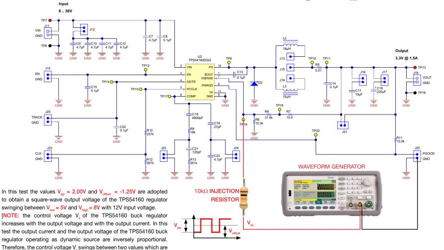
Figure 15. TPS54160 board operating as dynamic load
