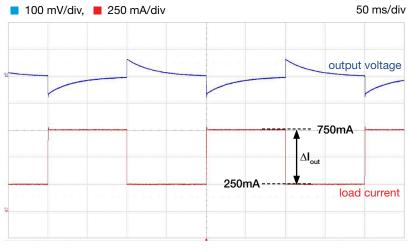
Figure 21. Load-transient operation, V<sub>in</sub>=5V, I<sub>out</sub>=250mA $\leftrightarrow$ 750mA, C<sub>ff</sub> ON, C<sub>out</sub>=C<sub>3</sub>=100µF, 100mΩ
