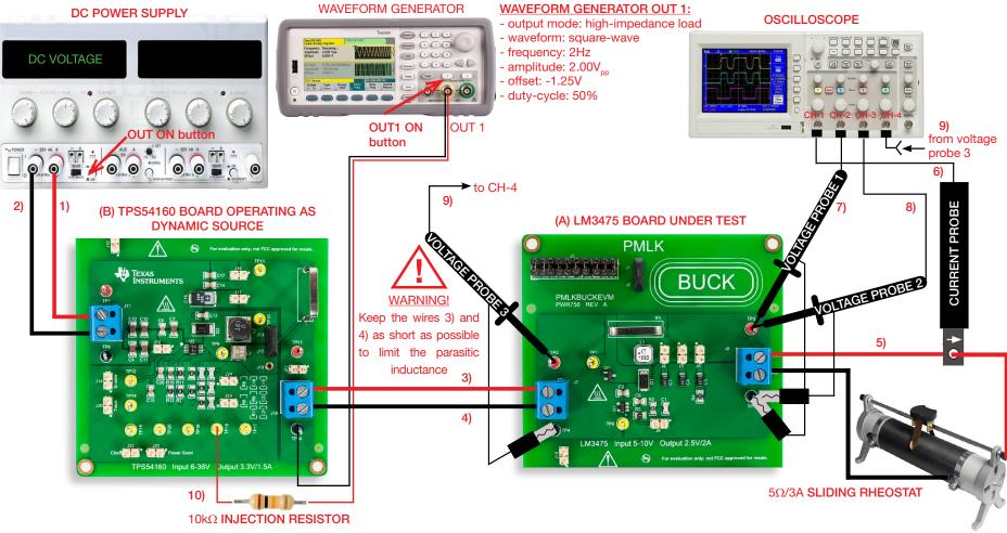
Figure 14. Experiment set-up.
