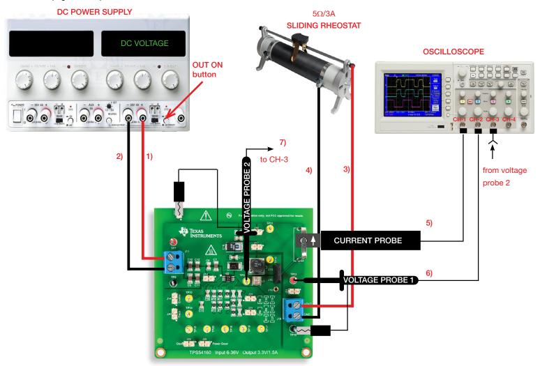
Figure 9. Experiment set-up.
