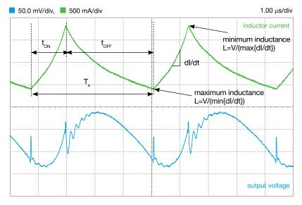
Figure 13.  $V_{in}$ =12V,  $I_{out}$ =1.9A,  $f_s$ =250kHz, L = L<sub>2</sub> = 18µH (ferrite inductor)
