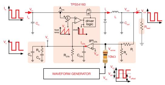
Figure 7. TPS54160 board operating in dynamic load emulation mode
