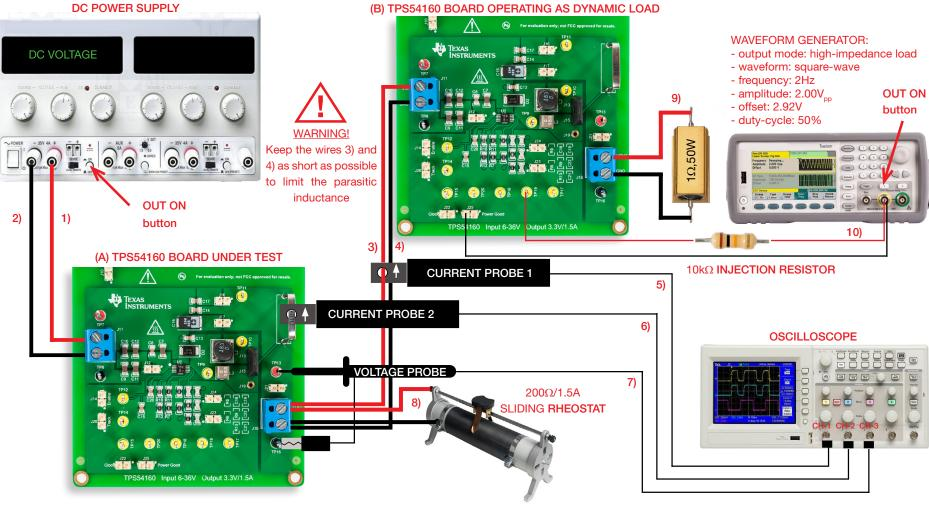
Figure 5. Experiment set-up.
