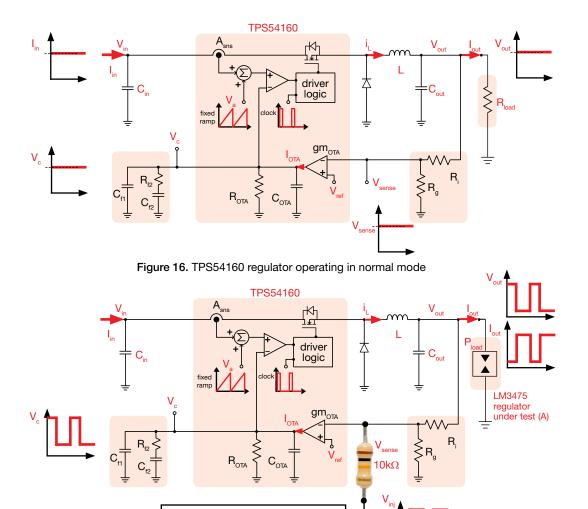
Figure 17. TPS54160 regulator operating in dynamic source emulation mode (B) feeding the LM3475 regulator under test (A)
