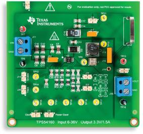
Figure 8. TPS54160 buck board: jumpers set-up for Test#2
