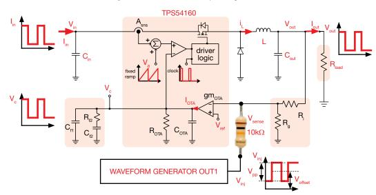
Figure 8. TPS54160 board operating in dynamic load emulation mode
