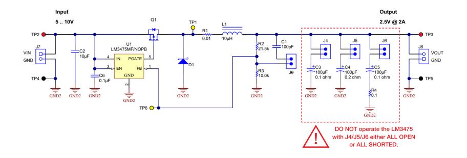
Figure 1. Circuit schematic of TI-PMLK LM3475 buck regulator
