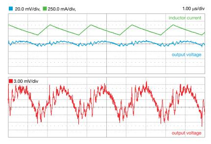
Figure 11.  $V_{in}$ =12V,  $I_{out}$ =0.15A,  $f_s$ =500kHz, L= L<sub>2</sub> = 18µH (ferrite inductor)
