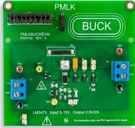
(a) LM3475 buck regulator under test
