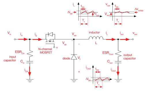
Figure 1. Buck converter simplified schematic
