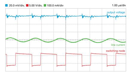
Figure 5. V<sub>in</sub>=6V, I<sub>out</sub>=1.5A, f<sub>s</sub>=500kHz, C<sub>out</sub>=220µF (electrolytic capacitor)
