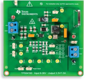
Figure 7. TPS54160 buck board: jumpers set-up for Test#1
