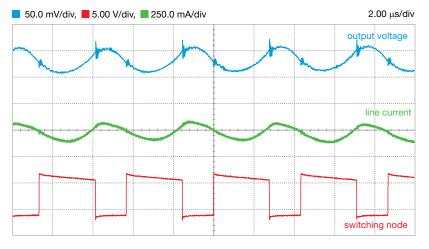
Figure 8.  $V_{in}$ =6V,  $I_{out}$ =1.5A,  $f_s$ =250kHz ,  $C_{out}$ =10 $\mu$ F (ceramic capacitor)
