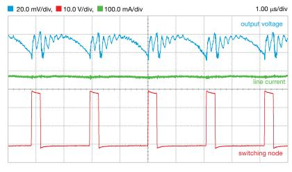
Figure 7.  $V_{in}$ =24V,  $I_{out}$ =0.4A,  $f_s$ =500kHz,  $C_{out}$ =10 $\mu$ F (ceramic capacitor)
