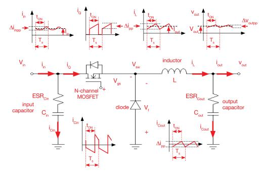
Figure 1. Buck converter simplified schematic
