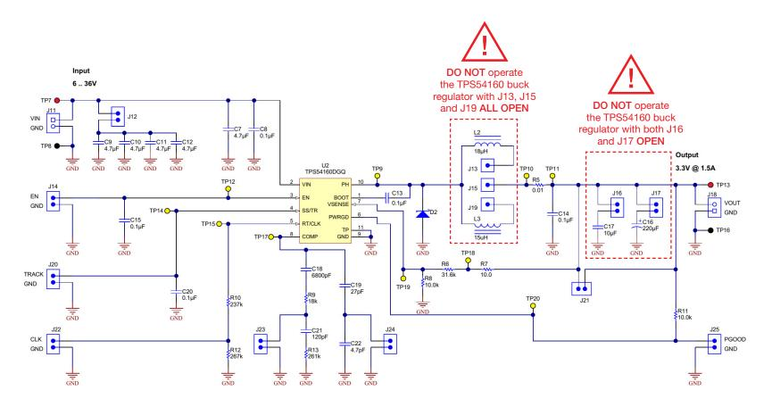
Figure 3. Circuit schematic of TI-PMLK TPS54160 buck regulator
