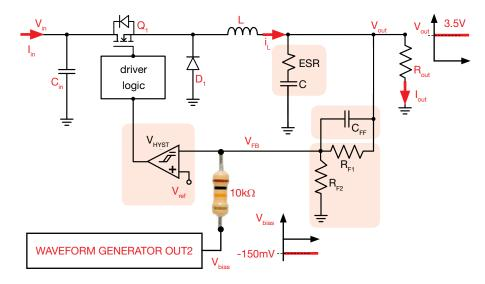
Figure 12. LM3475 board operating in dynamic load emulation mode
