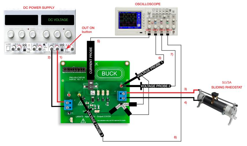
Figure 4. Experiment set-up.
