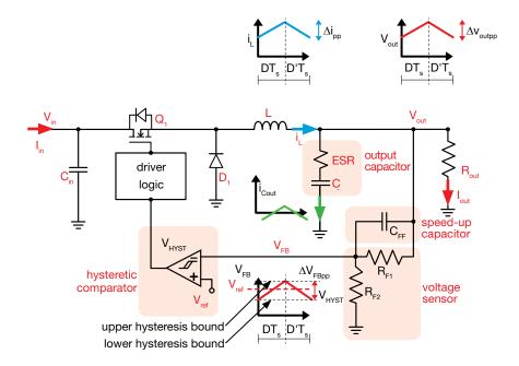
Figure 1. Simplified circuit schematic of LM3475 buck regulator
