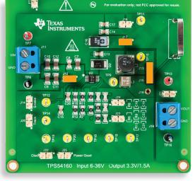
Figure 10. TPS54160 buck board: jumpers set-up for Test#2
