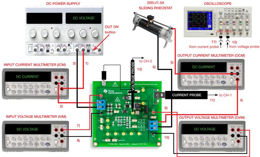
Figure 2. Experiment set-up.
