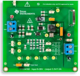
Figure 4. TPS54160 buck board: jumpers set-up for Test#2
