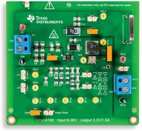
Figure 8. TPS54160 buck board: jumpers set-up for Test#1
