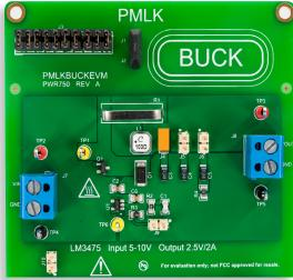
(a) LM3475 buck regulator under test
