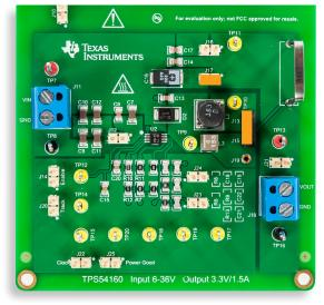
Figure 3. TPS54160 buck board: jumpers set-up for Test#1
