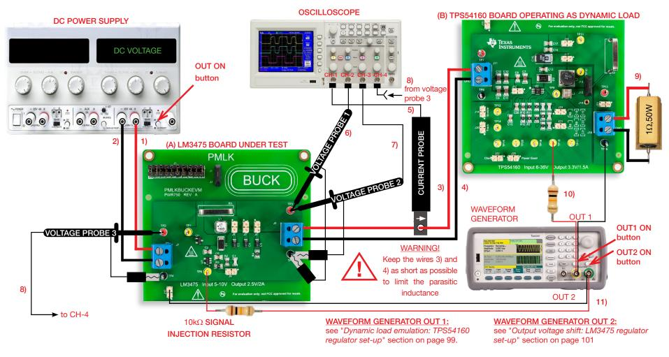
Figure 6. Experiment set-up.
