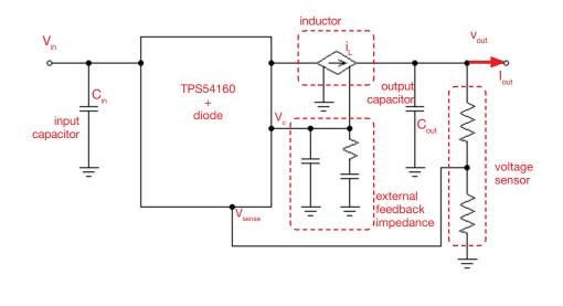
Figure 1. Simplified schematic of the TPS54160 buck regulator
