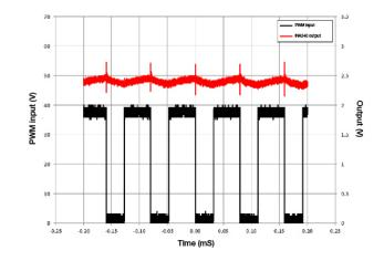
Figure 2. INA240-SEP output vs. PWM input
