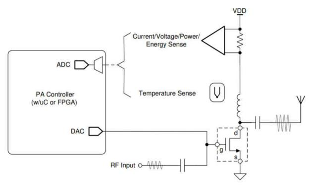
Figure 2. System protection configuration
