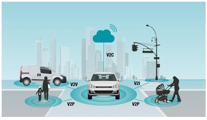
Figure 1. V2X Includes Vehicle-to-cloud (V2C), Vehicle-to-infrastructure (V2I), Vehicle-to-pedestrian (V2P) and Vehicle-to-vehicle (V2V) Connectivity
