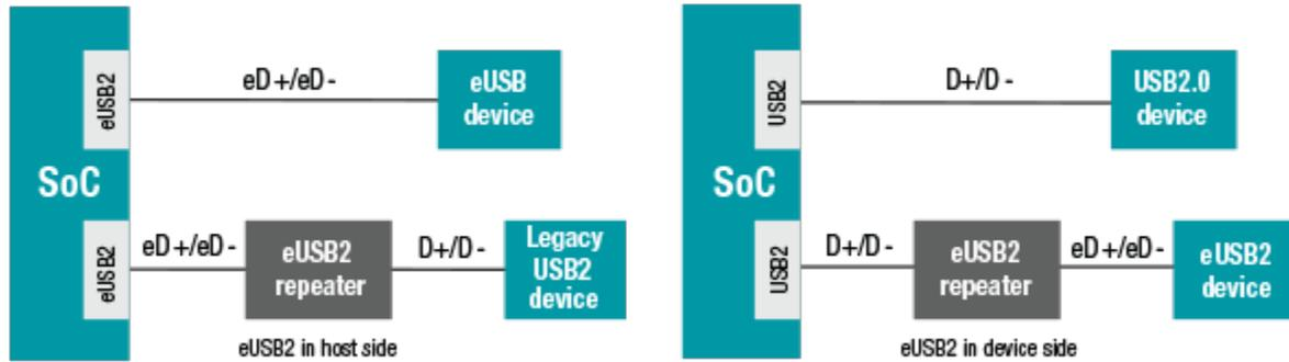
**Figure 1. eUSB2 applications using an eUSB2 repeater, such as the TUSB2E22**
