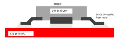
Figure 2. Typical Leaded Package CTE vs. Typical PCB CTE
