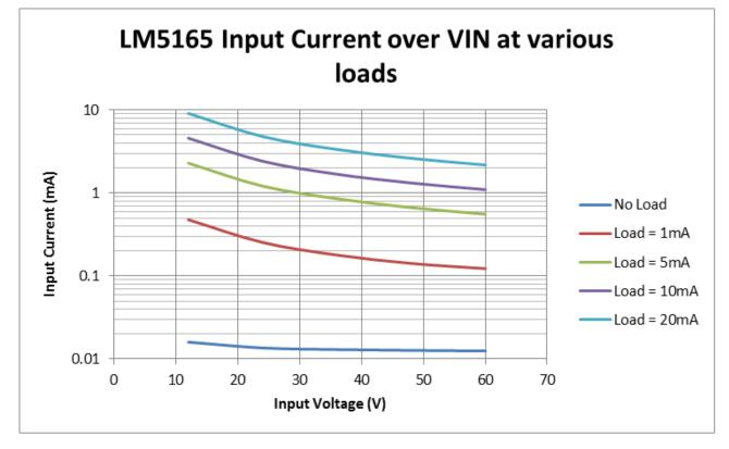
Figure 1 shows the input current data for an LM5165 DC/DC converter over the input voltage and load current ranges.
