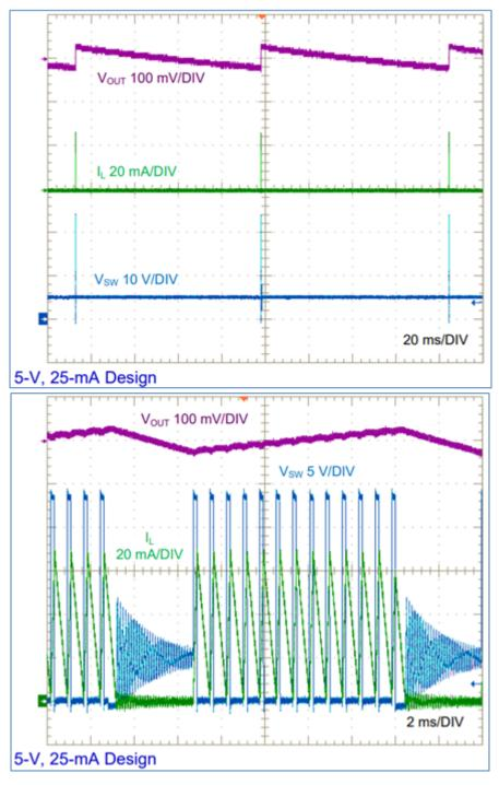
Figure 2. Switching Waveform at No Load (a); and a 25mA Load (b)
