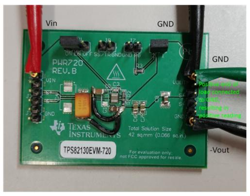
Figure 6. TIDA-01457 Connected as an Inverting Buck-boost Converter
