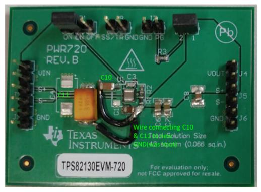
Figure 5. TPS82130EVM-720 Completely Modified to an Inverting Circuit
