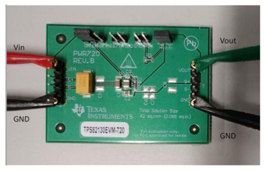
To begin, Figure 1 shows the standard EVM as it would be connected as a step-down converter.
