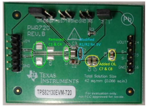
Figure 4. TPS82130EVM-720 Partially Modified to an Inverting Circuit
