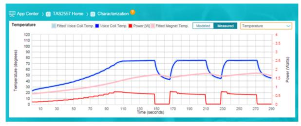
Figure 1. Speaker Coil Heating Time Constant
