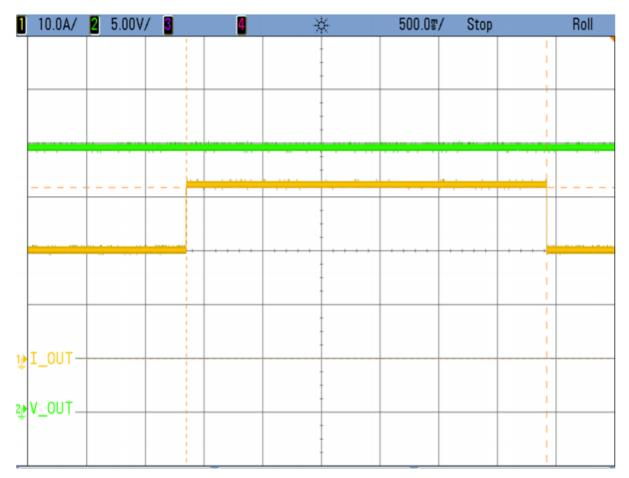
Figure 1. Short-time Overload Functionality of the TIDA-01494 Reference Design
