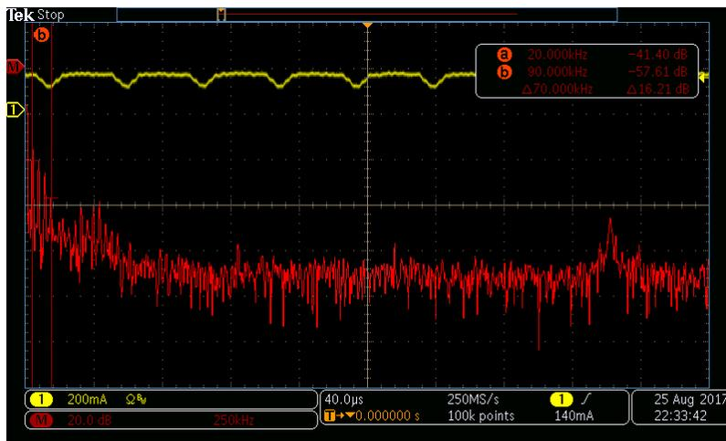
Figure 4. FFT of a 1.8V Load Current
