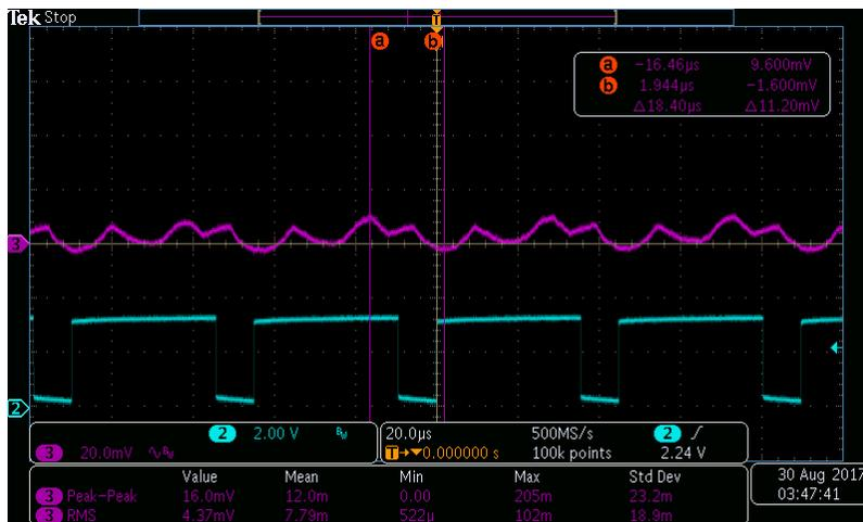
**Figure 6. 2.8V Voltage Ripple without Ferrite Bead – 11.2mV<sub>P-P</sub>**
