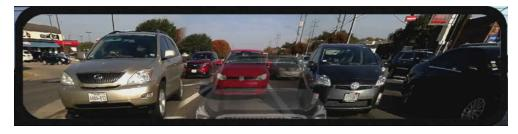
Figure 2. Rear-stitched View Panorama (RSVP) Display, with Virtual Vehicle Graphic Overlay for Relative Positioning
