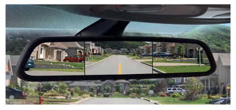
Figure 1. Three-camera Mirror replacement/CMS Example
