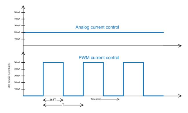
Figure 2. Analog and PWM Current Control
